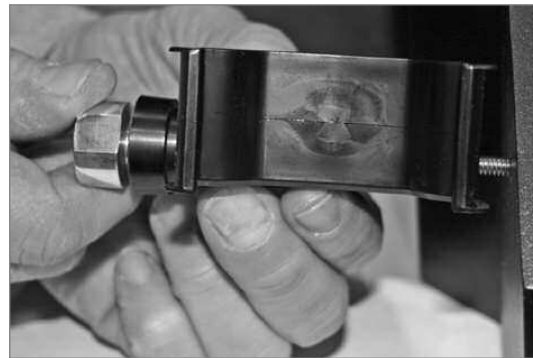
Fig. B: Thread the bolt through the wide end of the clamp and into the base of the RCX telescope.
