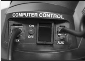
Fig. 13: Connect Autostar to the HBX port and Smartfinder to AUX port.
