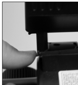
Fig. 9: Press down on the quick release tab to detach the viewfinder from the bracket.
