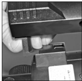
Fig. 8: Slide viewfinder into slip-fit bracket.
