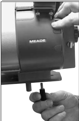
Fig. 7: Secure optical tube to the mounting plate using the mounting lock knobs.
