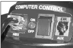
Fig. 12: Connect Autostar to the HBX port.
