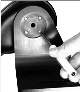
Fig. 6: Attach the mounting plate.
