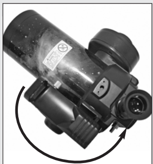
Fig. 24 [top view]: Rotate the telescope tube counterclockwise until it stops.
