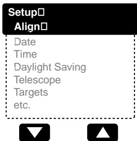
Fig. 27b: Menu options display on the second line. Use the Scroll keys to move up or down through the list of options. Press ENTER to select the desired option.
