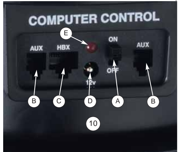
Fig. 2 (Inset): Computer Control Panel. (A) On/Off switch; (B) Auxiliary ports; (C) Handbox port; (D) 12v connector; (E) Power indicator light.
