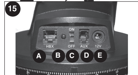
Fig. 1c (Inset): Computer Control Panel. (A) Handbox port; (B) Power indicator light, (C) ON switch; (D) Auxiliary port; (E) 12v Power.
