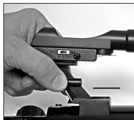
Fig. 9a: Slide viewfinder into slip-fit bracket.
