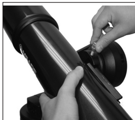
Fig. 7: Attach Vixen-style dovetail to mounting arm.
