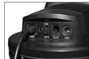
Fig. 13: Connect AudioStar to the HBX port.
