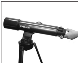
Fig. 8: Balance the optical tube.
