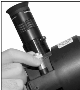
Fig. 10: Insert eyepiece and focus.
