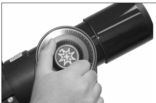
Step 2: Loosen vertical lock to move optical tube.
