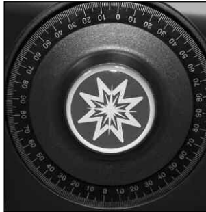
Fig. 28: Declination setting circle.
