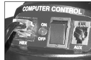
Fig. 12: Connect Autostar to the HBX port.
