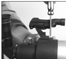
Fig. 8a: Attach the viewfinder bracket to the refractor optical tube assembly.
