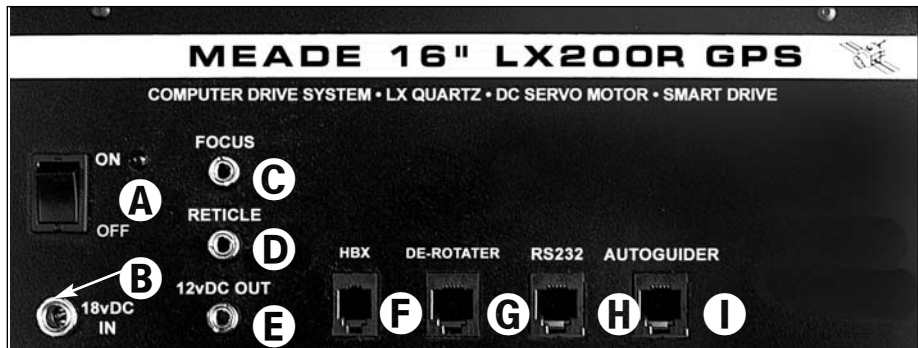
Figure 47: 16" LX200R Computer Control Panel.
