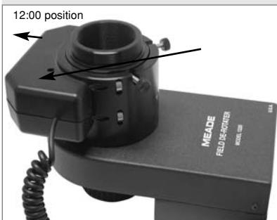
Fig. 63: Place the microfocuser over the adapter ring. Notice the orientation of the microfocuser.
