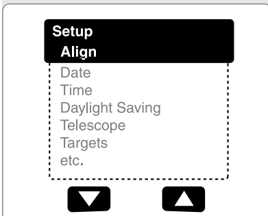
Fig. 17: Menu options display on the second line. Use the Scroll keys to move up or down through the list of options. Press ENTER to select the desired option.
