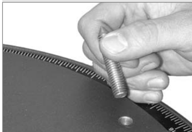
Fig. 51: Remove the pointed bolts from the drive base.
