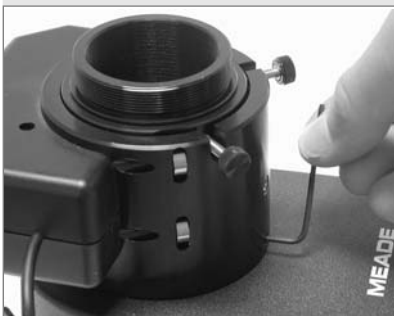
Fig. 64: Tighten the three microfocuser hex screws to a firm feel.
