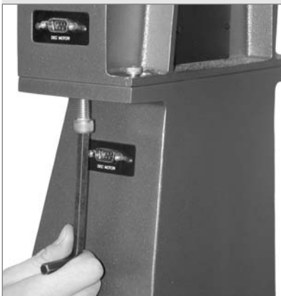
Fig. 57: Tighten the fork arm assembly using the provided hex key.
