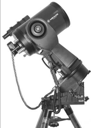
Fig. 44: LX200R mounted on an equatorial wedge.
