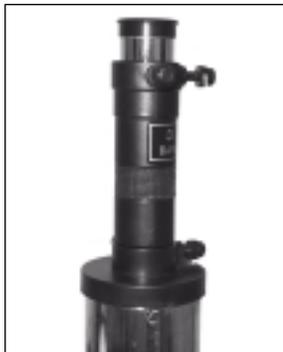
Fig. 15: Eyepiece and Barlow lens.
